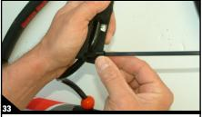
Slide the other small 8 mm wide piece of tubing over the zap strap.
