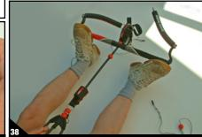
Test the Punch-Out by pulling on the trim loop, while forcing the bar with your feet.
