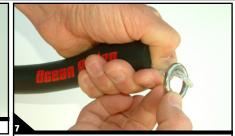
Insert the short piece of 10 mm wide tubing into the hole on the end of the bar winder. Repeat on the other side.
