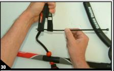
Pass the zap strap through the opening in the folded webbing at the bottom of the shock. The smooth side of the zap strap should face the outside of the shock.
