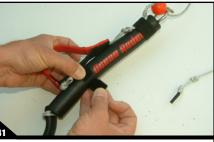
Attach the leader with grab handle to the screened red side float, secure with the Velcro tabs.
