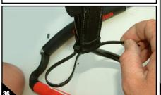
Pass the loose end of the zap strap through the opening in the folded webbing.
