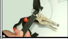
Push the shock down so it clears the D-ring and is sandwiched between the ring and the loop as shown.
